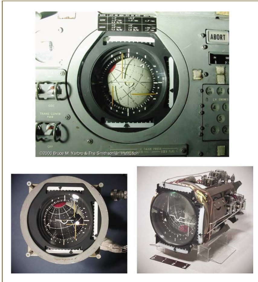
FIGURE 2.7 Assorted images of the Apollo flight director attitude indicator (FDAI), with gimbal lock limits of spacecraft orientation marked as red disks at the poles (near yaw equal to 0 degrees or 180 degrees). (From http://history.nasa.gov/ap08fj/09day3_green.htm , www.space1.com/Artifacts/Apollo_Artifacts/FLOWN_FDAI/flown_fdai.html , and www.space1.com/Artifacts/Apollo_Artifacts/FDAI/fdai.html .)
