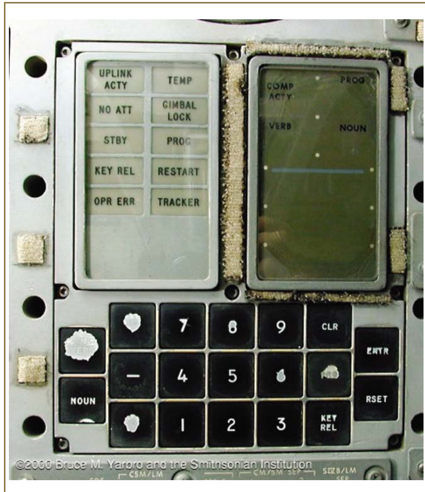
FIGURE 2.6 The actual Apollo 13 guidance computer console with “Gimbal Lock” warning light. (Source: http://history.nasa.gov/afj/pics/dsky.jpg from http://history.nasa.gov/afj/compassay.htm .)
